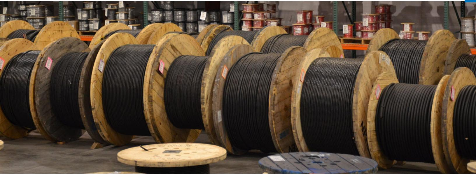
Tray cable can be used in many different types of cable tray systems, ranging from fixed wiring within buildings to hazardous locations and factory floors.
